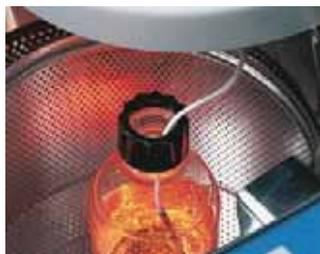
**Pt 100 Sensor.** 2<sup>nd</sup> Probe for reading sample temperature.
